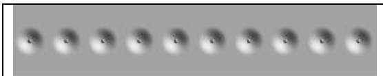
Figure 6a: Sun-illuminated view of the terrain ensonified (1000m long by 200m wide). Source lies to the centre left, elevated 500m above the surface. Each 5m deep, 80m wide depression has a 5m high, 10m wide knoll at its centre.
