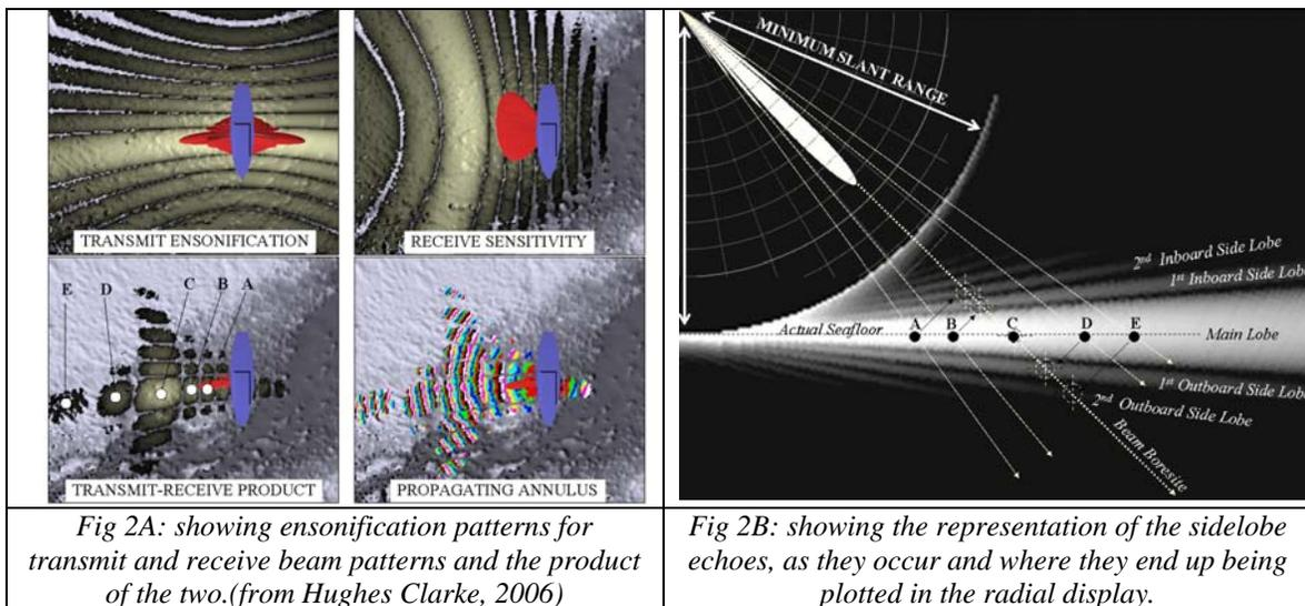
This will produce an apparent “halo” effect along the true seafloor. The width of the central band of echoes around the true seabed location will reflect the length of the projected main lobe beam footprint at that location. Beam spacing tighter than the 3dB limits will not significantly improve the achievable angular resolution of the image.
