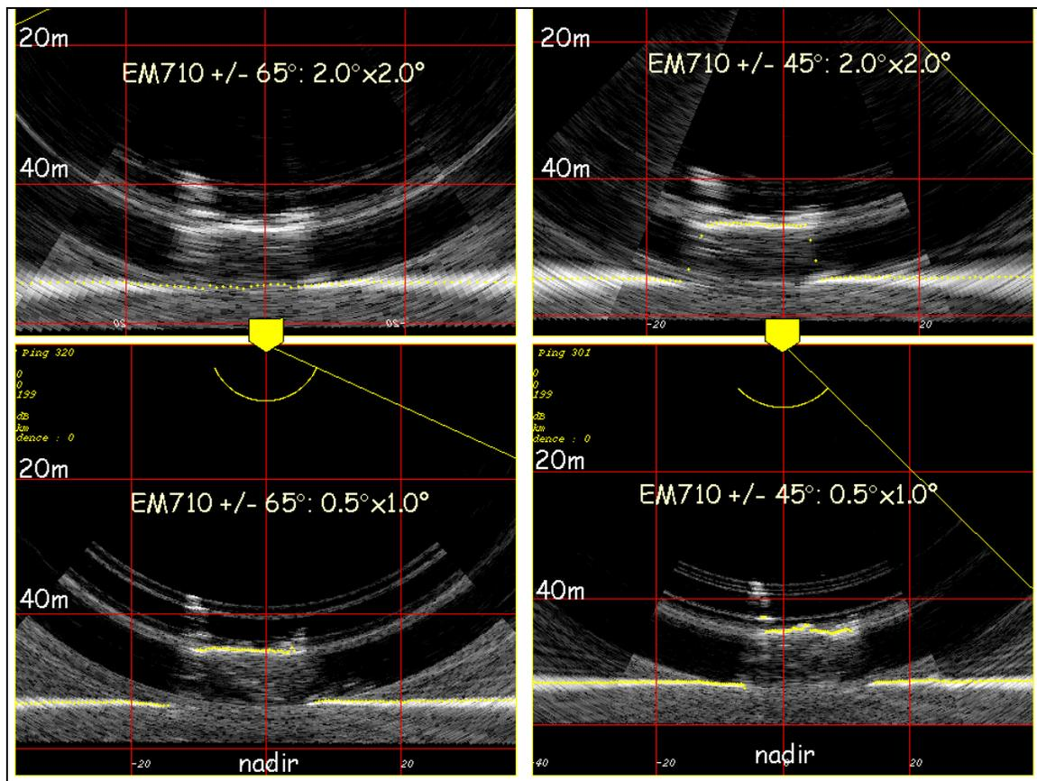
Figure 4: Four cross-section images located in almost the identical slice across the MV British Freedom. The upper two images were obtained using the 2.0°x2.0° version of the EM710. The lower two images were obtained using the 0.5°x1.0° version of the EM710. Angular sectors of +/-65° and +/-45° were used.
