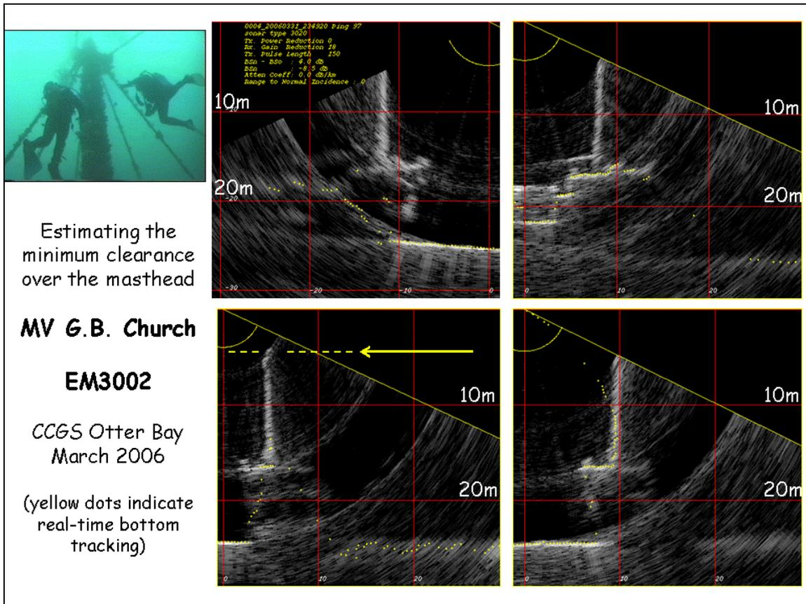
Figure 3: showing 4 instantaneous water-column images of the ping that best ensonified the mast of the G.B. Church. Note that in all geometries, there are faint echoes beyond the mast illustrating that complete beam occlusion never occurs.
