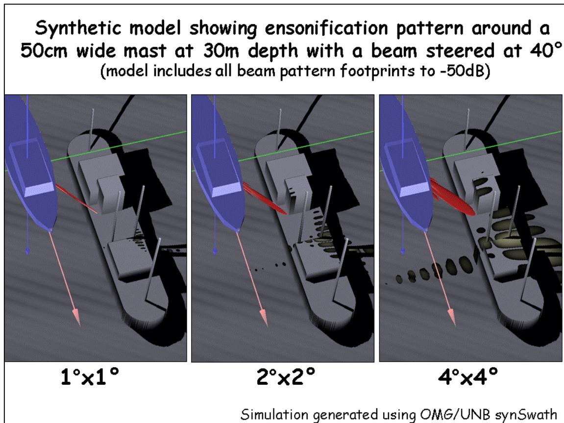
*Figure 1: simulation showing the full ensonification pattern of 1°, 2° and 4° beams on a wreck with typical dimension (30m depth, 50cm diameter mast with a beam steered at 40°). Note, the illustrated main lobe footprint is drawn to the first null, NOT to the 3dB limits and thus appears significantly wider.*
