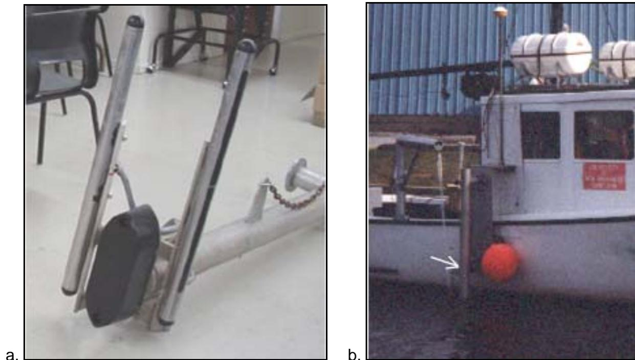
Figure 2: Retractable pole housing three Knudsen transducers (a) and the deployment of the pole on the UNB research vessel *Mary-O* (b).
